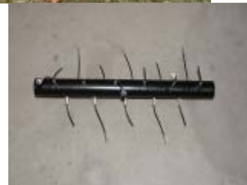
Ripper reel for tough-headed compositae species such as Echinacea , Silphium , Rudbeckia & Helianthus
